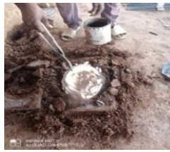
Plate 1: Showing a Successfully Cast Aluminum Plate Being Lifted out of the Mould by the Craft Man and the Researcher Respectively Using Pincer to lift it up.
