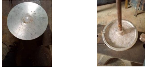
Plate 6: Already machined wheel head, treaded at the top, drilled and bolted to the shaft head.
