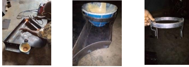
Plate 3b: Welding of flat bars to the top edge of the tray for the attachment of wood and an adjustable ring using flat bar constructed for the side placement for water container.
