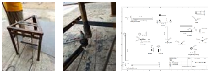
Plate 5: Foot pedal frame, the crank arm link of the pedal frame
