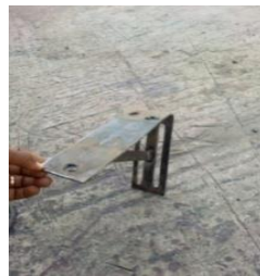
Plate 4. Bent and adjustable metal plate for the seat frame
